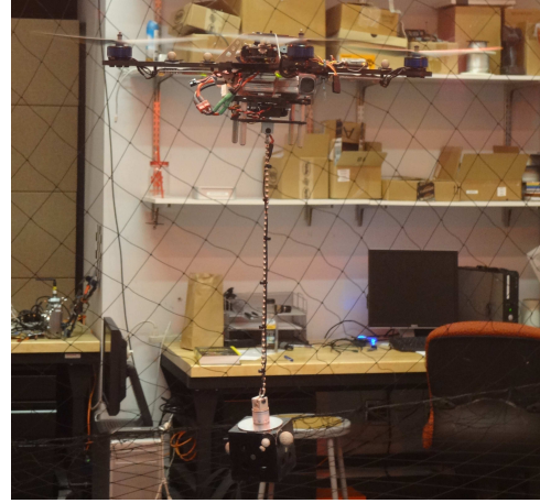
Fig. 6: Hummingbird quadrotor with cable-suspended load
